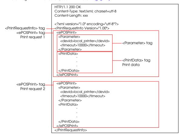
**Note:** Enclosing the <ePOSPrint> tag in the <PrintRequestInfo> tags enables sending multiple print requests to the printer.
