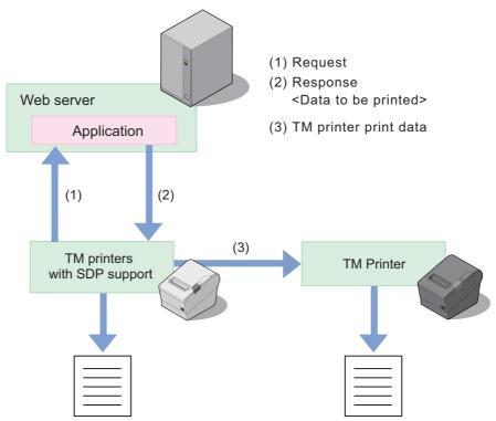
A TM printer with SDP support periodically sends a print request ((1) in the figure above) to the Web server. The Web server application includes print data in the response ((2) in the figure above) to a print request from the TM printers with SDP support. (When no print data exists, the Web server returns an empty response.)
