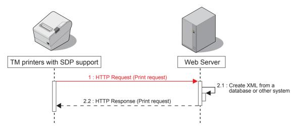
A TM printer with SDP support periodically sends a HTTP POST request (print request) shown below. The format of request message is URL-encoded form data (application/x-www-form-urlencoded). Set the sending destination and sending interval according to "Server Direct Print Settings" (p. 26). If communication fails, it is attempted again after a specified interval.
