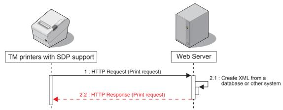
Response data created in XML(text/xml) from the application is returned. The data also contains print data. When an invalid print request is received, the server retries a request (print request) after a specified interval.
