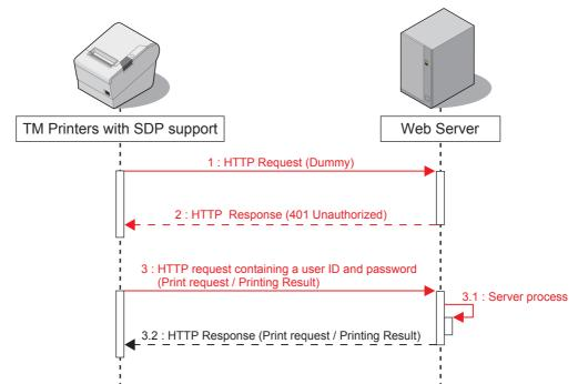
For Digest access authentication, the printer sends a dummy HTTP request before sending a print-related request to the server. The server returns a response with HTTP status code "401 Unauthorized". The printer sends a print-related request containing the user ID and password. The server carries out the Digest access authentication process. Once authenticated, the server continues to carry out the print-related process.
