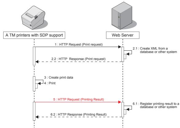
The application can check the printing result (if printing is properly finished) and the printer status by analyzing request data.
