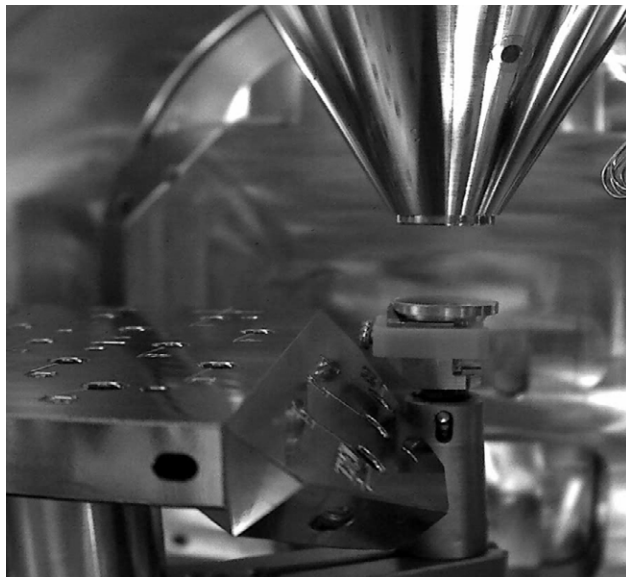
The pressure limiting aperture (PLA) is pre-mounted on the side of the multipurpose sample holder.
