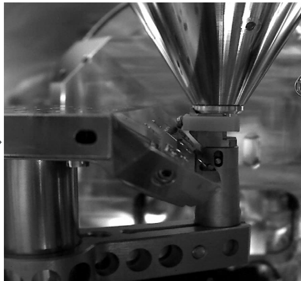
An automated routine moves the stage in order to insert the PLA when switching between high vacuum and low vacuum.
