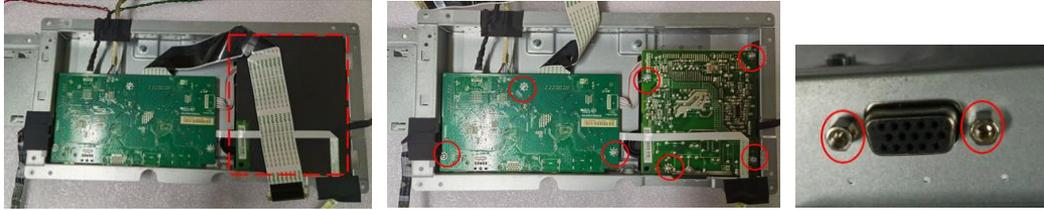
PCBA and Chassis separate step
