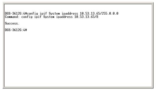
Figure 1-3. Assigning an IP Address
