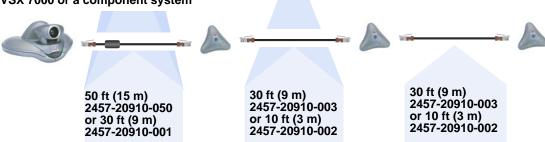
The ferrite bead must be at the end connected to the system.
