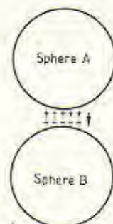
Fig. 5. As spheres A and B of 5(a) move together, \partial E/\partial t will change with time on the outer fringes until the total field is uniform as shown in 5(b), resulting in an increase in capacitance between spheres A and B.
