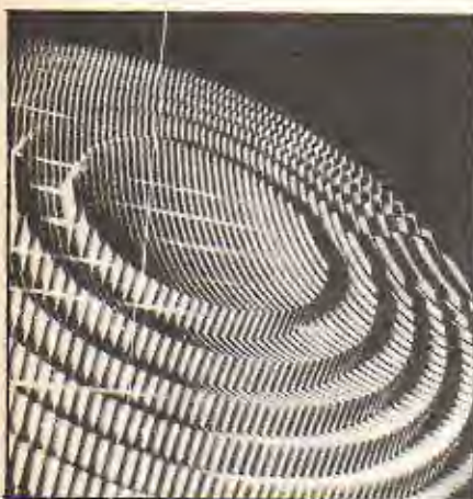
Fig. 1. One of the lens aerials constructed by the new method.
