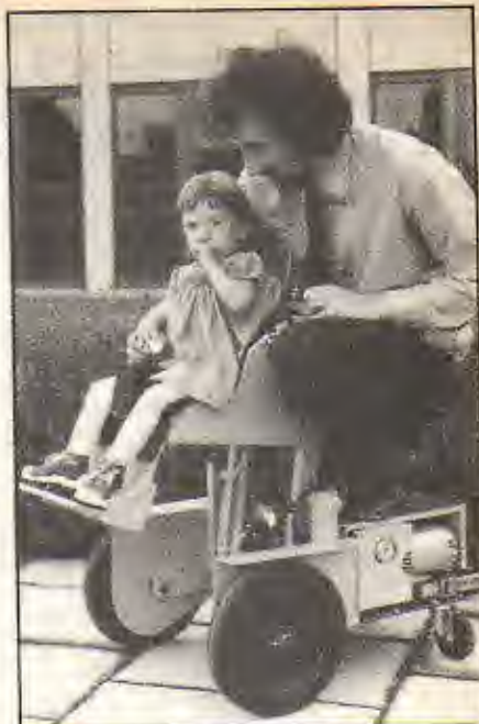
Ruth Everard, 19 months old, suffers from spinal muscular atrophy. She is seen here driving the wheelchair designed for her by her father, Dan Everard, who is perched behind. The design departs from standard practice by using shunt-wound motors controlled by c.m.o.s. to give free movement in three dimensions. The seat design is modular and can be made to fit any child; it can even be replaced with a standing platform. Its controls require very little strength to operate although the chair is capable of carrying an adult passenger, as shown. Ruth is learning to drive it about as quickly as most children learn to walk. The chair has been built in the labs of Cambridge Consultants Ltd. Dan once worked for CCL and the company have contributed laboratory space and engineering effort. In 1974 CCL developed a sensitive electronic wheelchair controller after working on a prototype wheelchair designed by his father for Terry Wiles, a thalidomide victim. That experience has now found another use in helping Dan with Ruth's chair.
