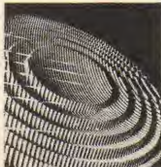
Front cover shows the millimetre-wave lens aerial of new construction described in this issue. Photo by Paul Brierley.
