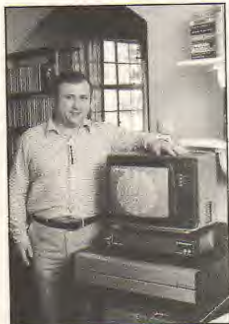
Mike Aldrich, managing director of Rediffusion Computers, with a Teleputer system, one of a range of videotex terminals that his firm believes will be at the centre of the 'home information system' towards the end of the 1980s. The terminals combine broadcast tv, videotex, video tape recorder, video disc and telecommunications with personal computers.
