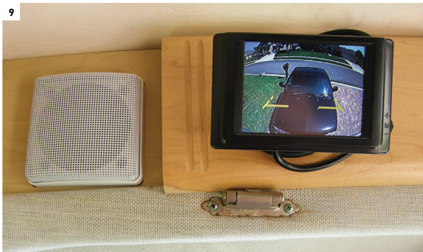
[7] A single hole was drilled through the base of the video monitor mount and the monitor mounted above the driver. [8] Enough slack was left in the cable to allow the cabinet door to open and close naturally without crimping it. [9] The monitor provides a crystal-clear view of the back of the motorhome when shifted into reverse.
