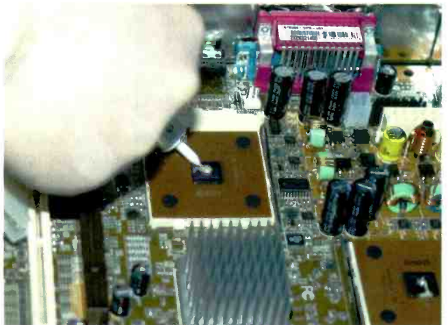
Photo 4. Silver compounds have been found to rival the heat dissipation of plain thermal greases that contain Zinc Oxide or silicone-based grease. Here, some Antec Silver is used to coat the CPU.
