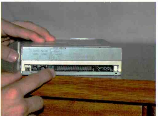
Photo 8. This detailed photograph shows the TEAC CD-RW being set to "Slave" mode. This is done so that the DVD burner can be set to "Master," decreasing the failure rate of expensive DVD mis-copies.
