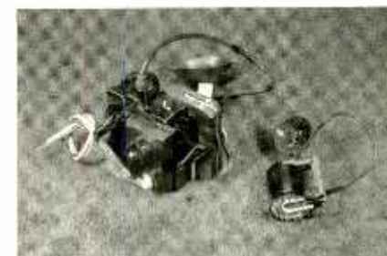
The flyback transformer pictured on the left is from a 21-inch monitor, while the one pictured on the right is from a 12-inch video terminal. Even smaller ones may be found in camcorders and mini-TVs.
