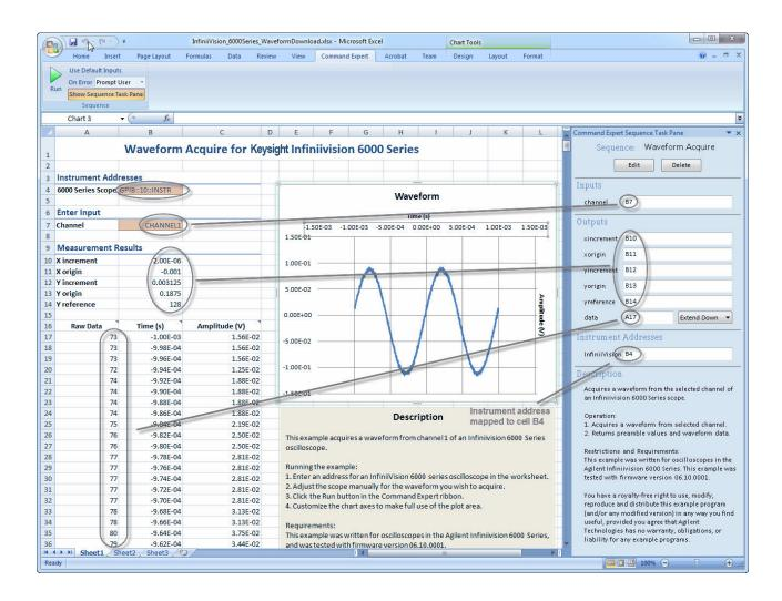
By entering the instrument address in cell B4, you can connect to the Infiniivision instrument. Now when you run the example, the sequence makes measurements on the specified channel, and writes actual instrument measurement results back to the workbook for analysis and display.
