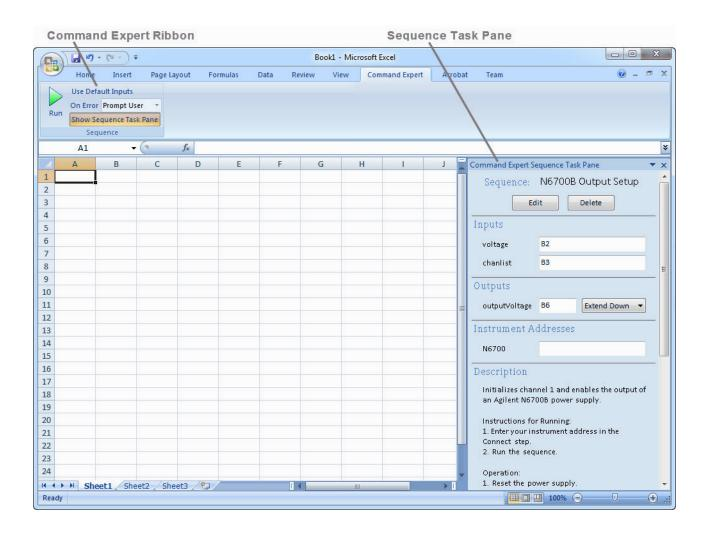
The Command Expert Ribbon contains high-level sequence settings and a Run button to run the sequence. Clicking the Show Sequence Task Pane button opens the Sequence Task Pane on the right side of the display.
