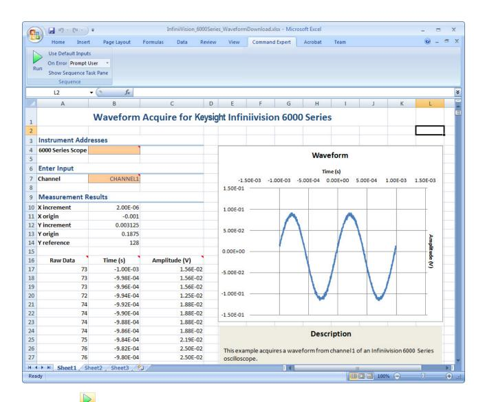
When you click the associated Command Expert sequence runs using input values from the workbook; for example, the Channel parameter. The sequence executes a number of instrument control steps, and writes measurement results back to the worksheet where they are displayed.
