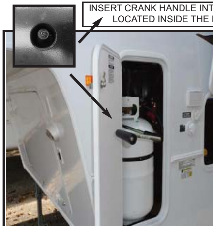
FIFTH WHEEL LANDING GEAR MANUAL OPERATION
