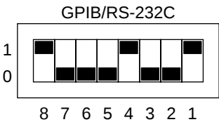
Fig. 5-2 GPIB Address 01001 Setting Example
