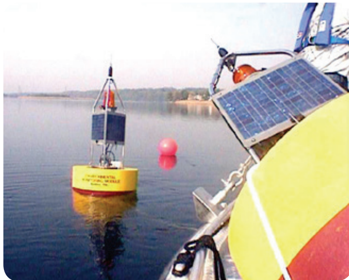
YSI Data Buoys deployed upstream of Sikorski Bridge.
