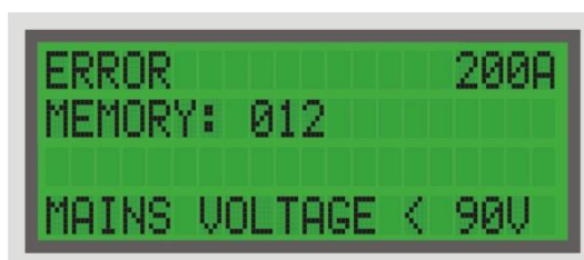
Figure 4-7: Error message "Mains Voltage < 90V"
