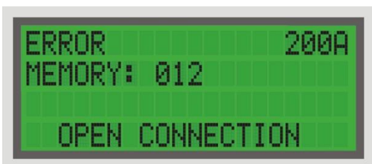
Figure 4-2: Disconnection of the current cables and corresponding error message
