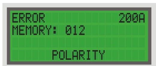
Figure 4-3: Error message "Polarity"
