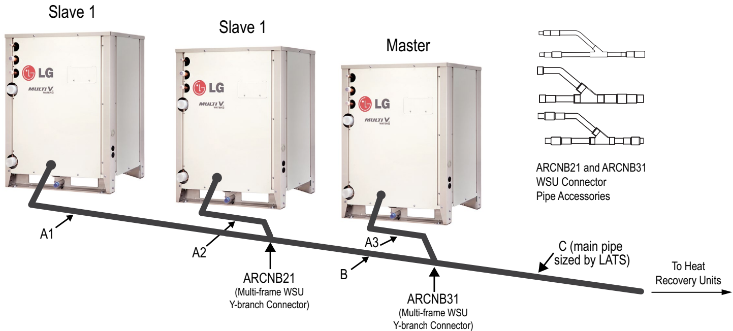
Figure 31: Heat Recovery Triple-Frame Connections.
