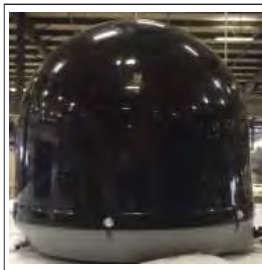
Figure 7-1: The dome satellite located on top of the coach can be raised, allowing easy access to change switches to a new satellite provider.
