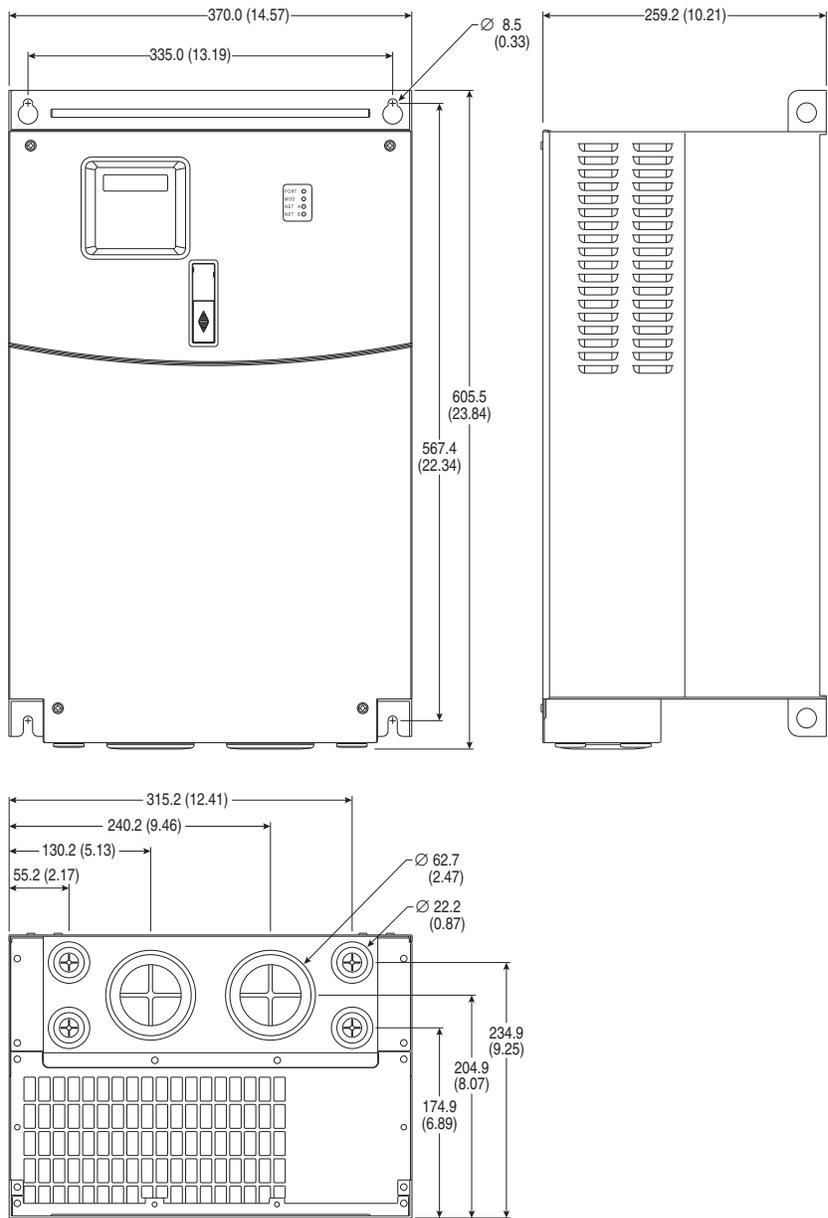
**Figure 21 - PowerFlex 400 Frame F Drive**
