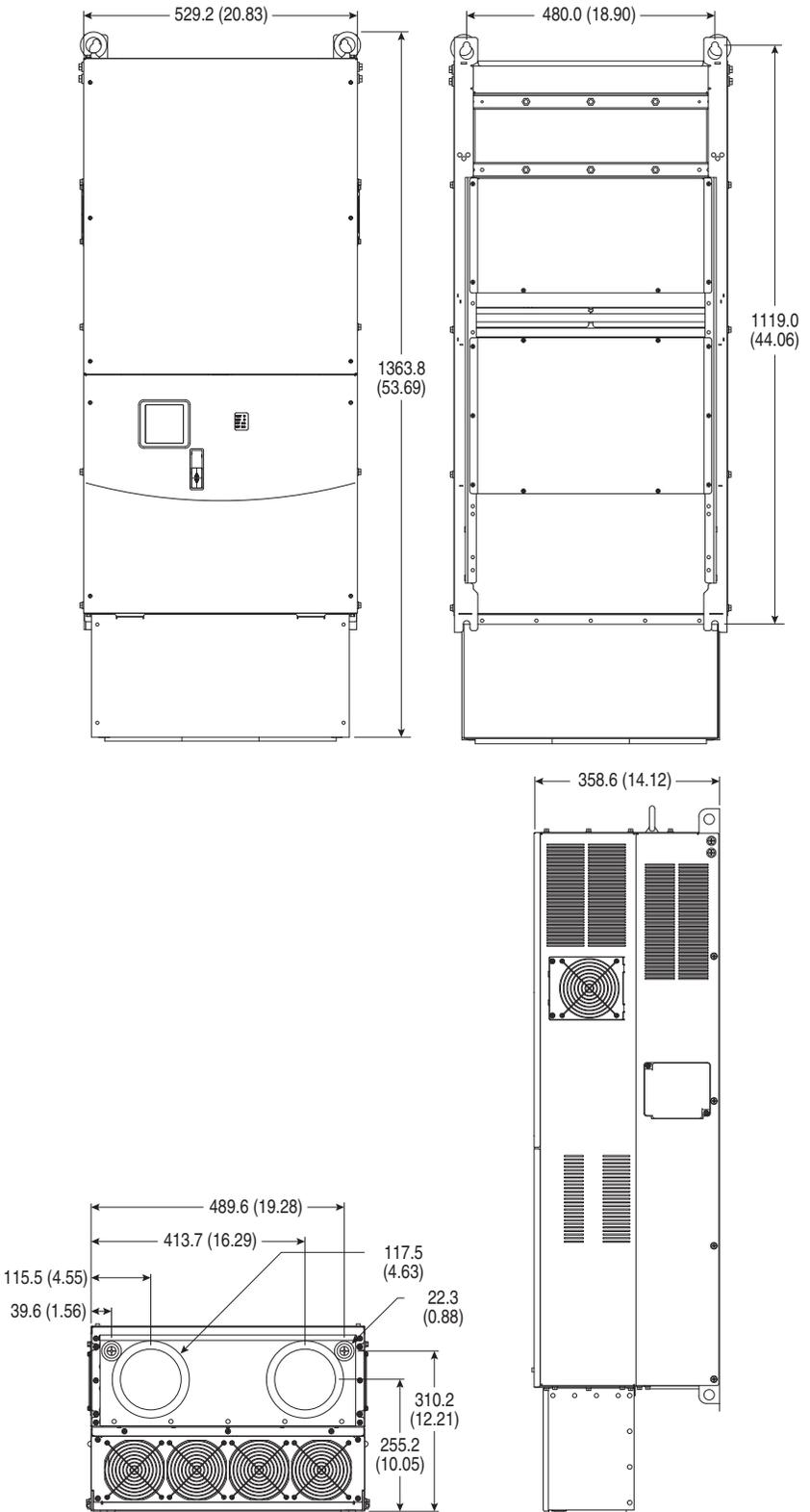
**Figure 24 - PowerFlex 400 Frame C Flange Mount Drive**
