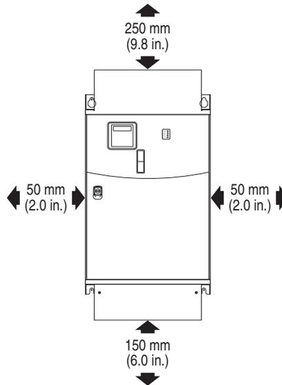
**Figure 4 - Frames G & H Mounting Clearances**
