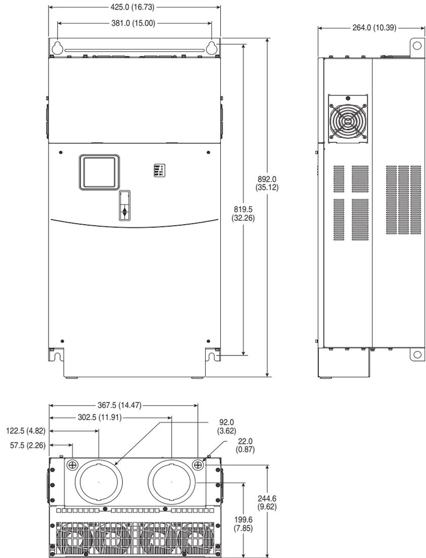
**Figure 23 - PowerFlex 400 Frame H Drive**
