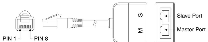
**Figure 31 - RJ45 Two-Position Terminal Block Adapter**
