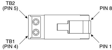
**Figure 32 - RJ45 Adapter with Integrated Termination Resistor**
