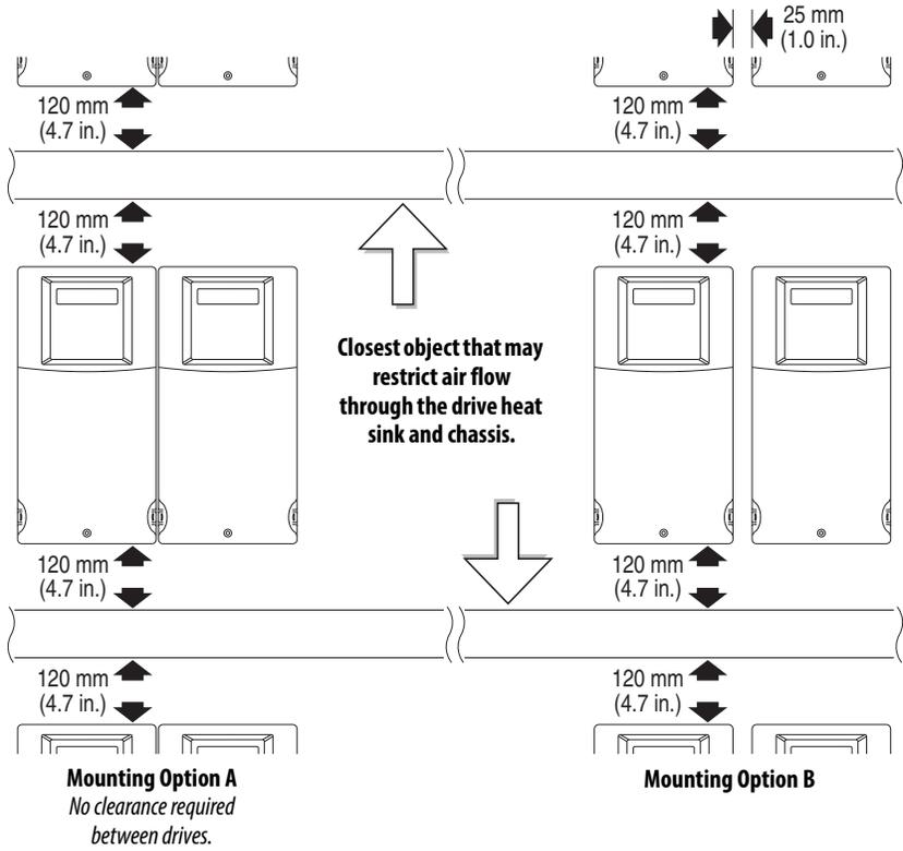
**Figure 2 - Frames D & E Mounting Clearances**
