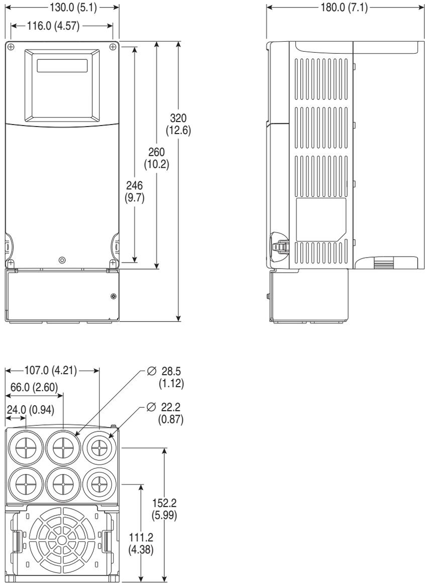
**Figure 19 - PowerFlex 400 Frame D Drive**
