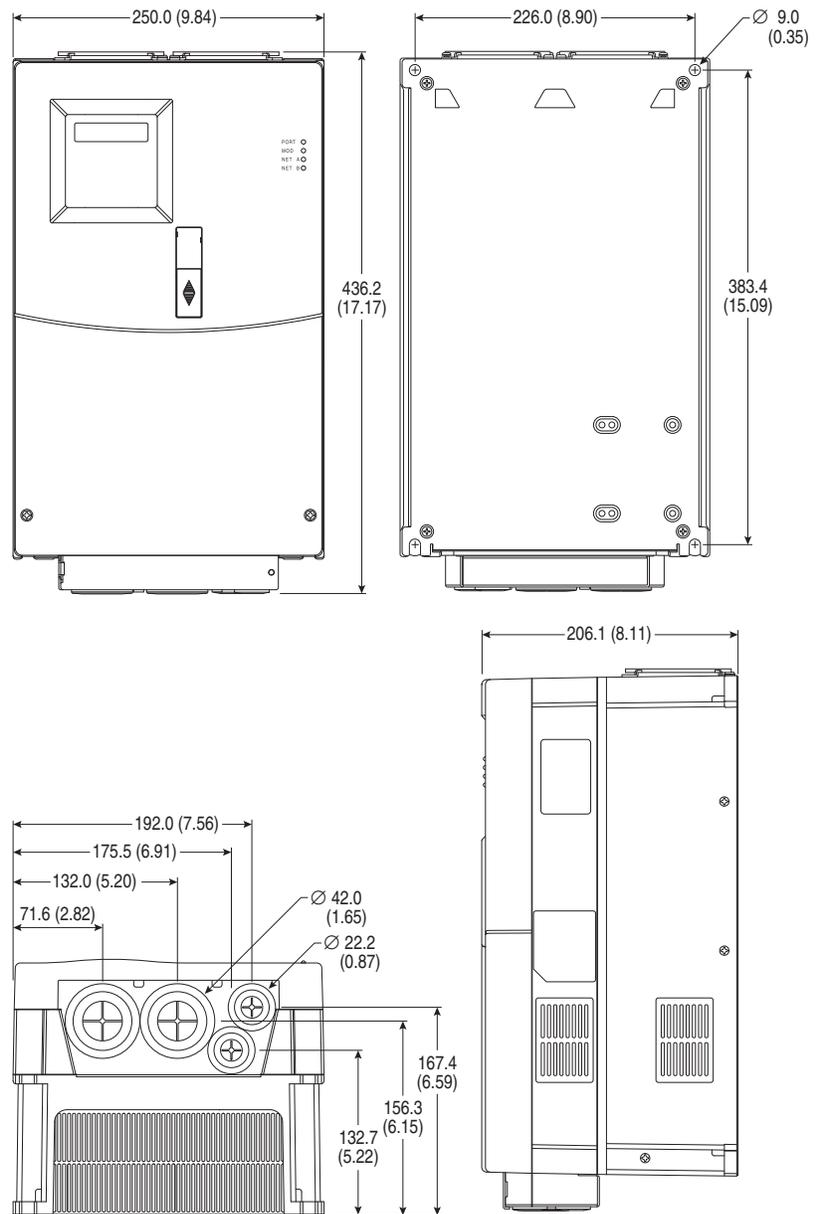
**Figure 20 - PowerFlex 400 Frame E Drive**
