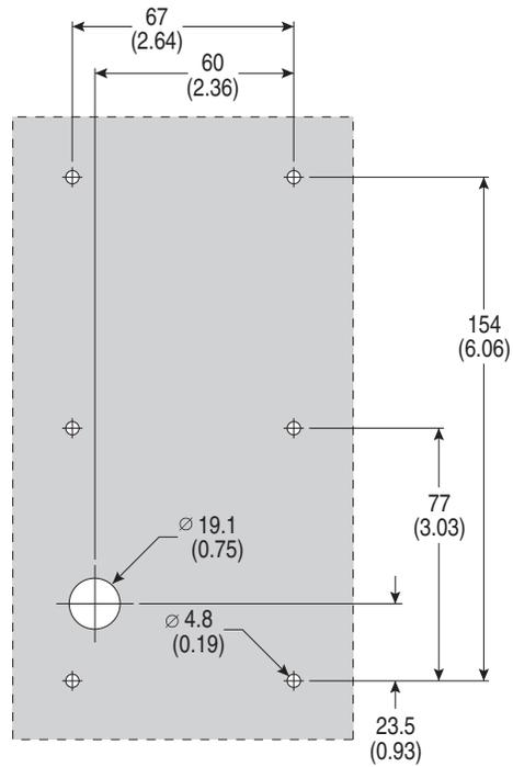
**Figure 29 - NEMA Type 1 Bezel**
