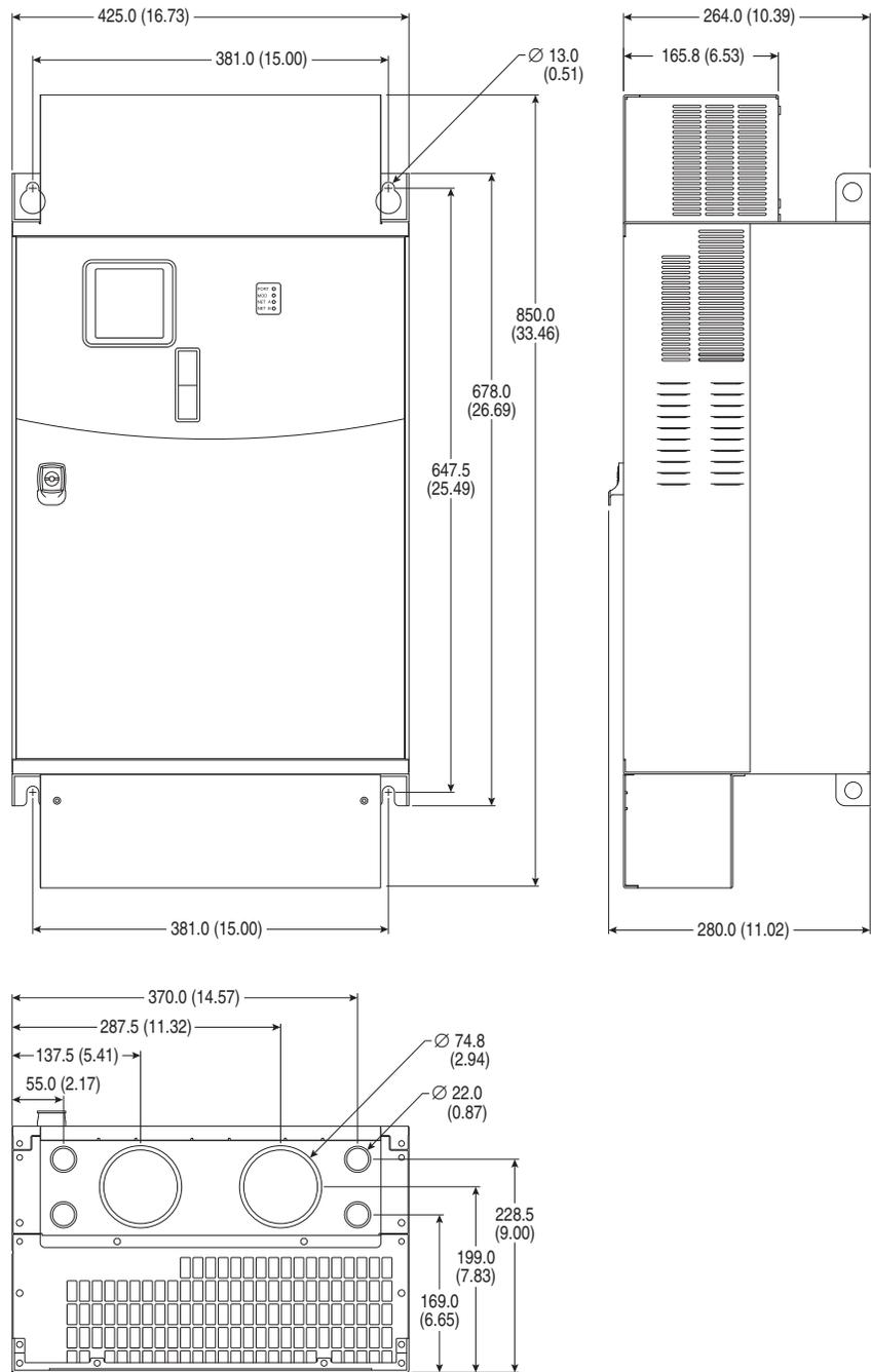
**Figure 22 - PowerFlex 400 Frame G Drive**
