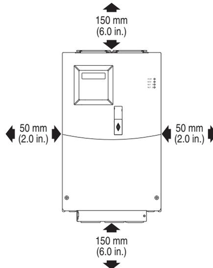
**Figure 3 - Frame F Mounting Clearances**
