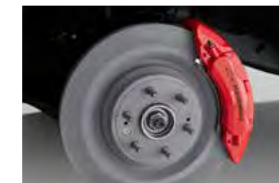
FRONT 6-PISTON BREMBO ® BRAKE UPGRADE SYSTEM IN RED, (PAGE 29).
