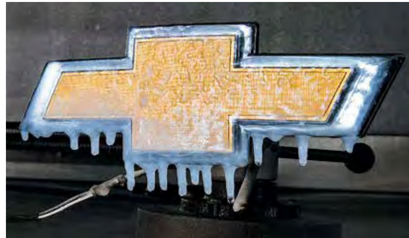
ILLUMINATED BOWTIE EMBLEMS ARE CYCLED 1.5 MILLION TIMES, FEATURE 100% WATERPROOF CONSTRUCTION AND ARE TESTED TO WITHSTAND EXTREME TEMPERATURES FROM -40°F TO 158°F.
