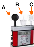
A. Globe thermometer B. Natural wet bulb thermometer C. Dry bulb thermometer
