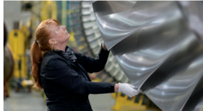
Vicki Lunsford helps build the heart of the first-ever 7HA.03 Gas Turbine, the rotor, for Florida Power & Light. Once installed, Gas Power's newest and highest-capacity gas turbine will help FPL squeeze more power from every cubic foot of natural gas, saving money and burning less fuel.
