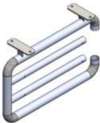
50 cm Antenna Bracket Design and Attachment for Wall Mounting
