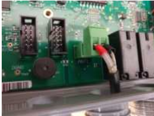
Figure 9 – Antenna Signal Cable Connectivity
