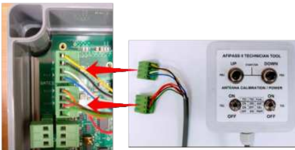
Figure 17 – Technician Tool Connections in AfiPass II Controller
