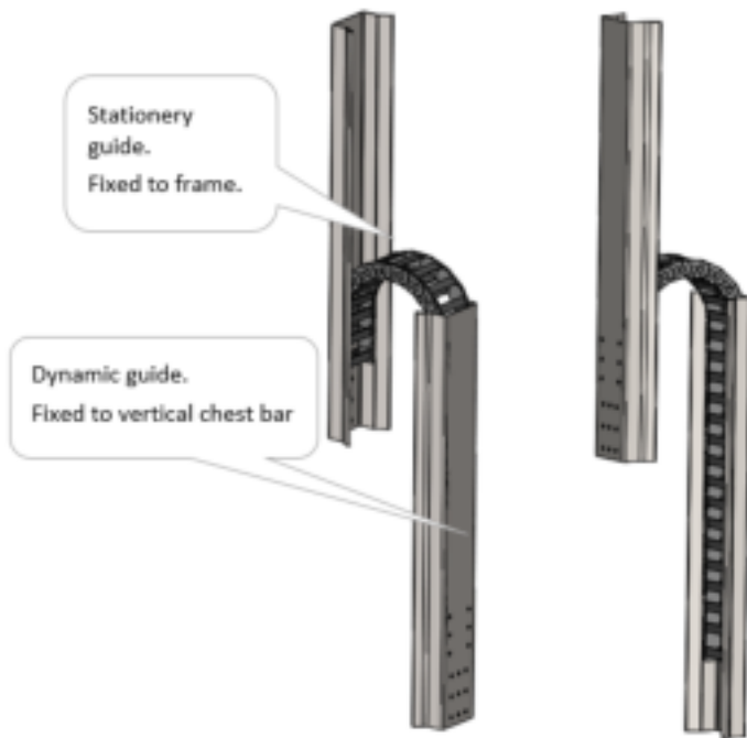
Both sides supported. Recommended for long life of cables
