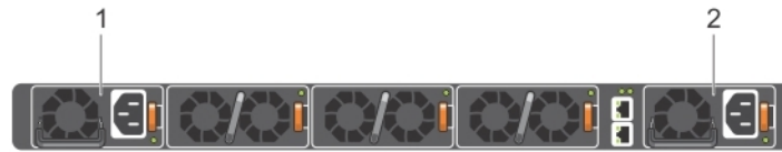
Figure 14 S4048-ON PSUs on the rear panel
