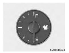
This gauge indicates the approximate amount of fuel remaining in the fuel tank.
