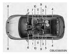
The SRS consists of the following components:
