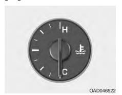
This gauge indicates the temperature of the engine coolant when the ignition switch is in the ON position.
