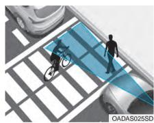
If there is a pedestrian(s) or bicycle(s) in between you and the vehicle in front, Leading Vehicle Departure Alert may not operate properly.
