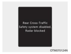
When the rear bumper around the rear corner radar or sensor is covered with foreign material, such as snow or rain, or installing a trailer or carrier, it can reduce the detecting performance and temporarily limit or disable Rear Cross-Traffic Safety system.
