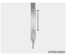
Pull the dipstick out again and check the level. The level should be between F and L.
