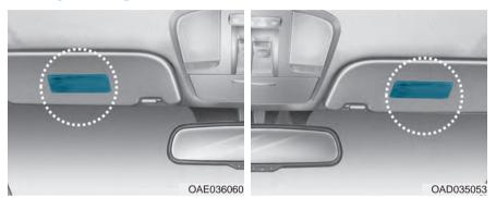
Air bag warning labels, required by the U.S. National Highway Traffic Safety Administration (NHTSA), are attached to alert the driver and passengers of potential risks of the air bag system. Be sure to read all of the information about the air bags that are installed on your vehicle in this Owners Manual.
