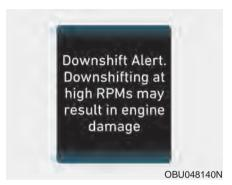
Downshift Alert. Downshifting at high RPMs may result in engine damage
