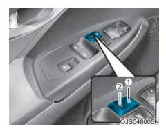
The driver side door armrest is equipped with a central door lock switch. The lock button is indicated by a (1) symbol. The unlock button is indicated by a (1) symbol.
