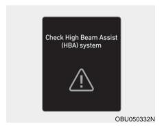
When High Beam Assist is not working properly, the 'Check High Beam Assist (HBA) system' warning message will appear and \(\frac{1}{2}\) warning light will illuminate on the cluster. We recommend that the system be inspected by an authorized HYUNDAI dealer.
