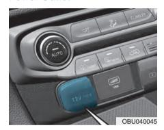
The power outlet is designed to provide power for mobile telephones or other devices designed to operate with vehicle electrical systems. The devices should draw less than 180 W with the engine running.
