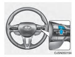
Press the Driving Assist to turn Cruise Control off. The Cruise (© CRUISE) indicator will go off. Always press the Driving Assist button to turn Cruise Control off when not in use.
