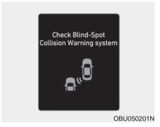
When Blind-Spot Safety system is not working properly, the 'Check Blind-Spot Collision Warning system' warning message will appear on the cluster, and the system will turn off automatically, or the system will be limited. We recommend that the system be inspected by an authorized HYUNDAI dealer.
