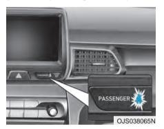
As a reminder to the front passenger, the front passenger's seat belt warning lights will illuminate for approximately 6 seconds each time you place the ignition switch to the ON position regardless of belt fastening. If you continue not to fasten the seat belt and you drive over 6 mph (9 km/h), the warning light will stay
