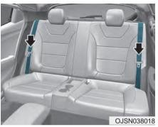
Move the seatbelt toward the outboard position before folding down the seatback to avoid the seatbelt system interfering with the seatback.
