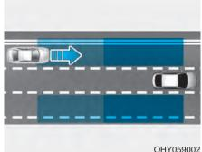
Blind-Spot Collision Warning helps detect and inform the driver that a vehicle is approaching at high speed from the blind spot area.
