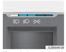
When engine is operating in a high rpm area, it is indicated by LEDs according to the corresponding engine rpm.
