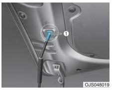
4. Pull out the support rod and hold the hood open with the support rod (1).
