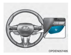
N mode or CUSTOM mode may be selected by pressing the N button. The system resets to be in the NOR-
