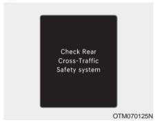
When Rear Cross-Traffic Safety system is not working properly, the 'Check Rear Cross-Traffic Safety system' warning message will appear on the cluster, and the system will turn off automatically, or the system will be limited. We recommend that the system be inspected by an authorized HYUNDAI dealer.
