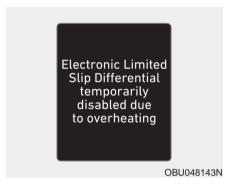
Electronic Limited Slip Differential temporarily disabled due to overheating
