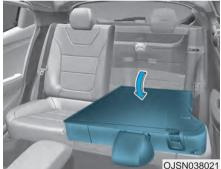
Remove the belt from the clip (1) and pull up the seatback folding lever (2), then fold the seat toward the front of the vehicle.
