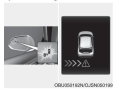
Rear Cross-Traffic Safety system will warn the driver when a collision is imminent.
