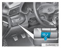
Turning the system On/Off (Blind-Spot Safety button)
