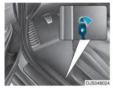
The fuel filler door is opened from inside the vehicle using the fuel filler door release lever.
