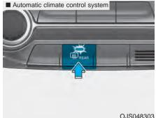
The defroster heats the window to remove frost, fog and thin ice from the interior and exterior of the rear window, while the engine is running.
