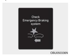
When Forward Collision-Avoidance Assist is not working properly, the 'Check Emergency Braking' system warning message will appear, and the and warning lights will illuminate on the cluster. We recommend that the system be inspected by an authorized HYUNDAI dealer.
