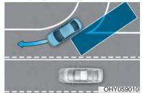
Blind-Spot Safety system may not operate properly when driving where the road merges or divides. The system may not detect the vehicle in the next lane.
