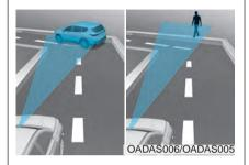
Forward Collision-Avoidance Assist may detect a vehicle, pedestrian in the next lane or outside the lane when driving on a curved road.
