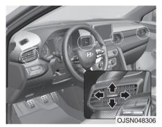
The instrument panel vent air flow can be directed up/down or left/right using the vent adjustment lever.
