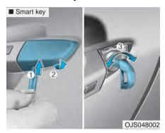
If you lock the driver's door with a mechanical key, all vehicle doors will lock.
