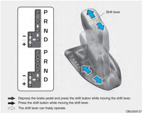
\* To move the shift lever from/to P (Parking) or between R (Reverse) and D (Drive), you must depress the brake pedal for the vehicle to stand still.
