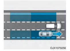
Blind-Spot Collision Warning helps detect and inform the driver that a vehicle is in the blind spot.
