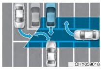
Rear Cross-Traffic Safety system may detect vehicles which are parking or pulling out near your vehicle (for example: a vehicle leaving beside your vehicle, a vehicle parking or pulling out in the rear area, a vehicle approaching your vehicle making a turn, etc.). If this occurs, the system may unnecessarily warn the driver.
