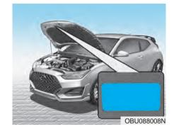
You can find out which air conditioning refrigerant is applied to your vehicle on the label located inside of the hood.
