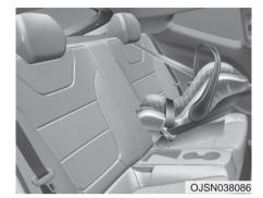
A rear-facing child seat provides restraint with the seating surface against the back of the child. The harness system holds the child in place, and in an accident, acts to keep the child positioned in the seat and reduce the stress to the neck and spinal cord.
