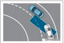
Blind-Spot Safety system may not operate properly when driving on the curved road. The system may recognize the vehicle in the same lane.
