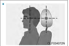
Adjust the head restraints so the middle of the head restraint is at the same height as the height of the top of the eyes.
