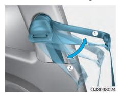
You can adjust the extension guide to allow easy access to the seat belt and for the rear seat passengers to easily enter and exit the vehicle.
