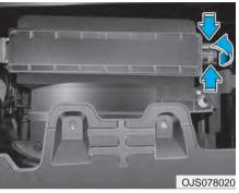
Remove the climate control air filter case while pressing the lock on the right side of the cover.
