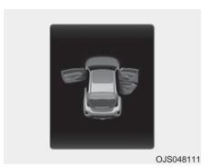
This warning is displayed if any door or the hood or the liftgate is left open. The warning will indicate which door is open in the display.
