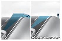
Forward Collision-Avoidance Assist may not detect other vehicles, pedestrians in front of you while driving uphill or downhill adversely affecting the performance of the sensors.
