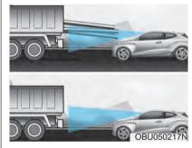
If the vehicle in front of you has cargo that extends rearward from the cab, or when the vehicle in front of you has higher ground clearance, additional special attention is required. Forward Collision-Avoidance Assist may not be able to detect the cargo extending from the vehicle.
