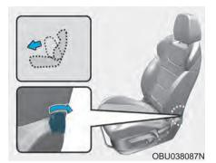
To get in or get out of the driver's door from the rear seat, the driver's seat should be folded by pulling the lever toward the rear of the vehicle.
