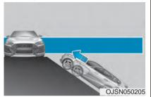
Rear Cross-Traffic Safety system may be limited when the vehicle is on a uphill or downhill slope, or near it, and may not detect the vehicle approaching from the left or right. If this occurs, the system may not warn the driver when necessary.
