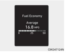
The trip computer mode displays information related to vehicle driving parameters including fuel economy, tripmeter information and vehicle speed.
