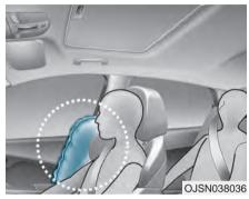
The purpose of the air bag is to provide the vehicle's driver and the front passenger with additional protection than that offered by the seat belt alone.
