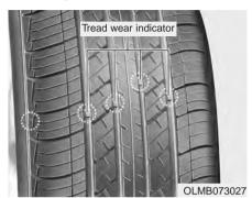
If the tire is worn evenly, a tread wear indicator will appear as a solid band across the tread. This shows there is less than 2/32 inch (1.6 mm) of tread left on the tire. Replace the tire when this happens.
