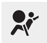
SRS warning light
