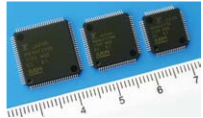
The second entry in the FM3 Family of new 32-bit microcontrollers uses ARM's Cortex™-M3 cores from ARM of Britain
