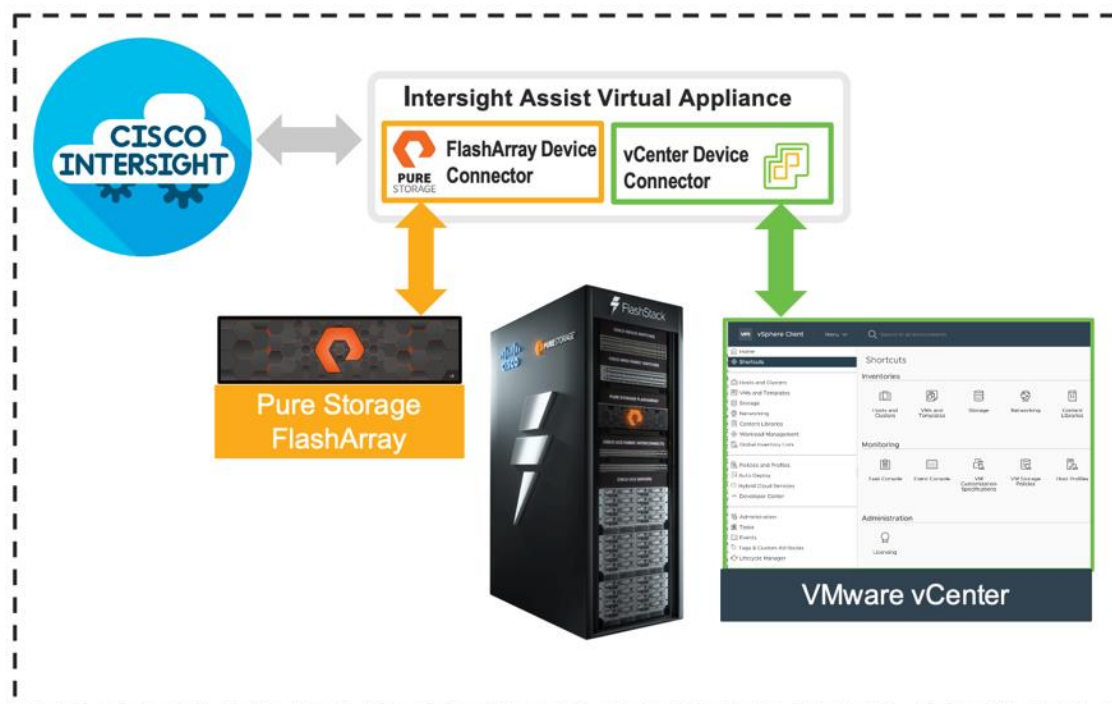
Figure 37. Managing Pure Storage FlashArray and VMware vCenter through Cisco Intersight using Intersight Assist
