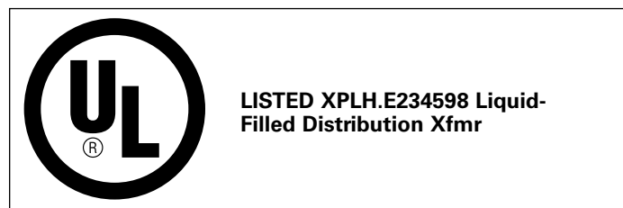
Figure B1 – Example transformer mark for a UL Listed ANSI-compliant transformer.
