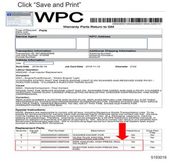
**Note:** When printing out the WPC shipping label, the label might indicate that the part is not hazardous as shown in the display picture. That indicator is based on a new or unused part. Any part that comes in contact with flammable liquid (i.e. fuel) is considered a hazardous material. Please review the shipping label
