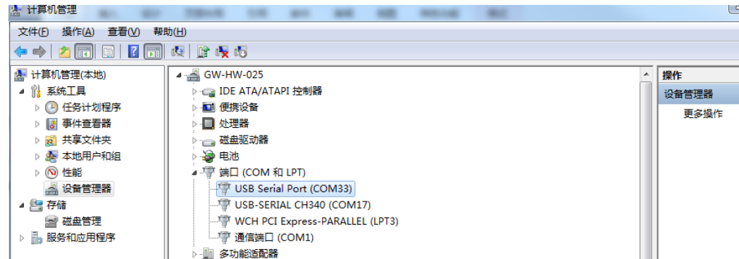
Figure 2-1 Driver Installed Information
