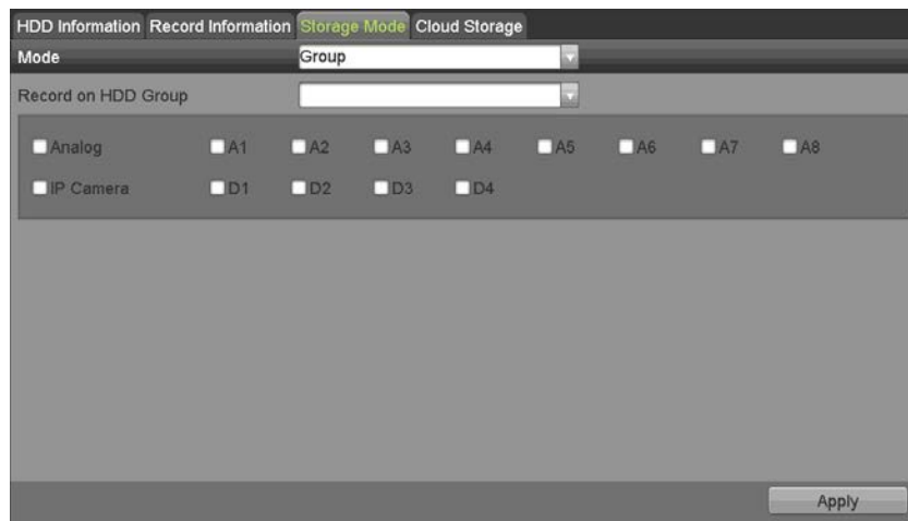
Figure 5-2 HDD - Storage Mode
