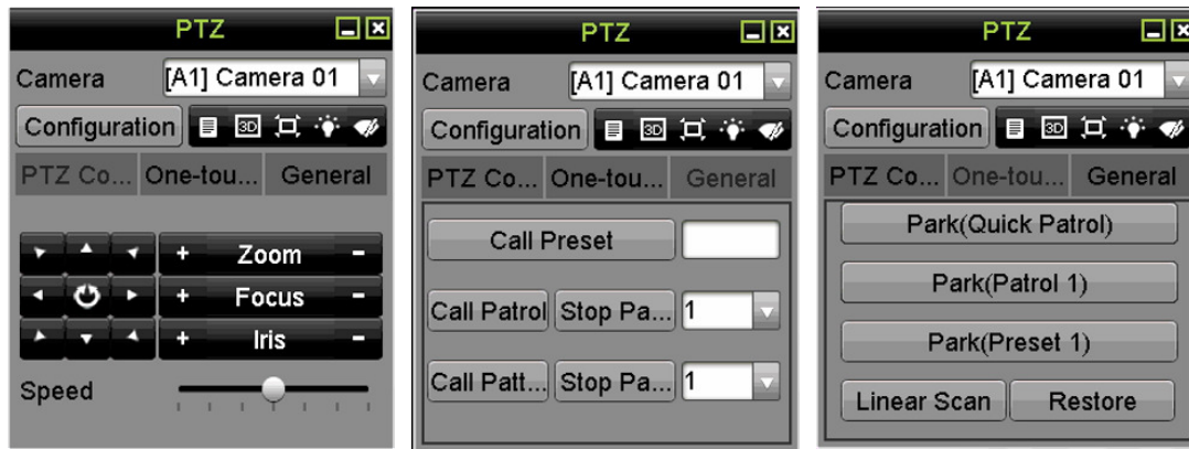
Figure 4-14 PTZ Control Panels
