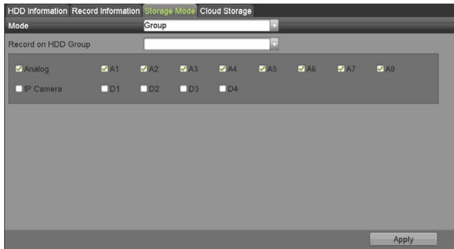
Figure 5-26 HDD Storage Mode
