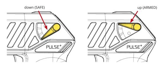
Ambidextrous safety switch can be operated from either side of the energy weapon.
