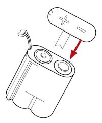
Reattach the battery pack to the device.The connectors make a click when they fit together.
