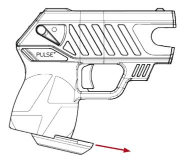
4 Pull the battery pack out of the energy weapon. Tapping the heel of the device on the leg or palm of the hand may help release the battery pack from the energy weapon.
