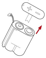
6 Remove the CR123 battery cells from the battery pack and replace them with new ones.
