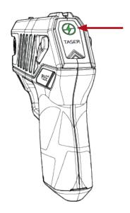
An orange LED indicates a "low" battery. In some conditions, especially low temperature ( $-4 \,^{\circ}\text{F}/-20 \,^{\circ}\text{C}$ ) the LED may display orange even if the battery has sufficient charge left.
