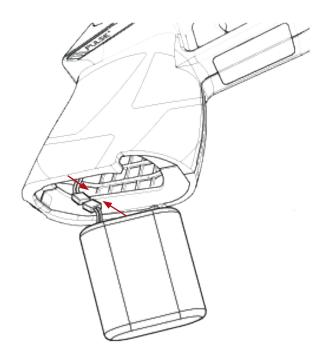
9 Push the battery into the battery well.
