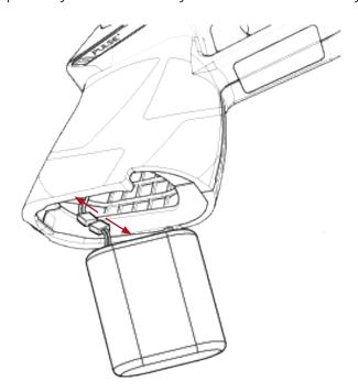
5 Place your fingers on the battery cap lid, and pry off the battery cap. It may help to squeeze the battery pack by the curved sides and then by the flat sides to loosen the lid.
