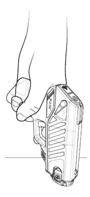
6 Confirm that the cartridge is secure by gently pulling on the sides of the cartridge.
