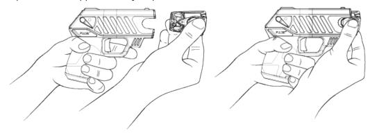
5 Gently press the cartridge against a firm, flat surface until it locks into place. Do not slam the energy weapon against the surface; doing so may damage the cartridge.
