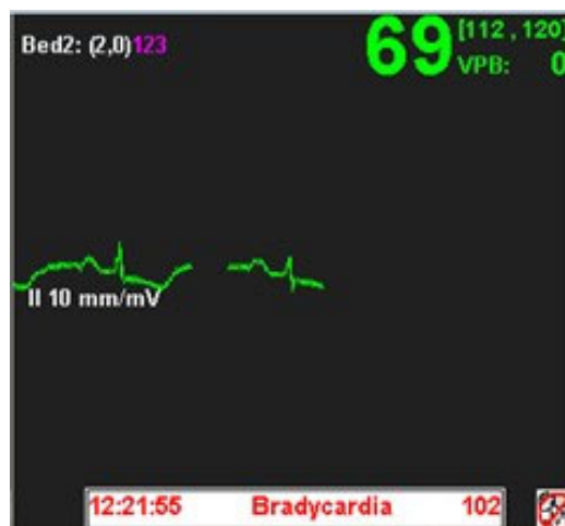
Figure 25 - Sub-screen showing the crossed-out printer icon in the lower right corner, indicating that automatic alarm printouts are disabled.
