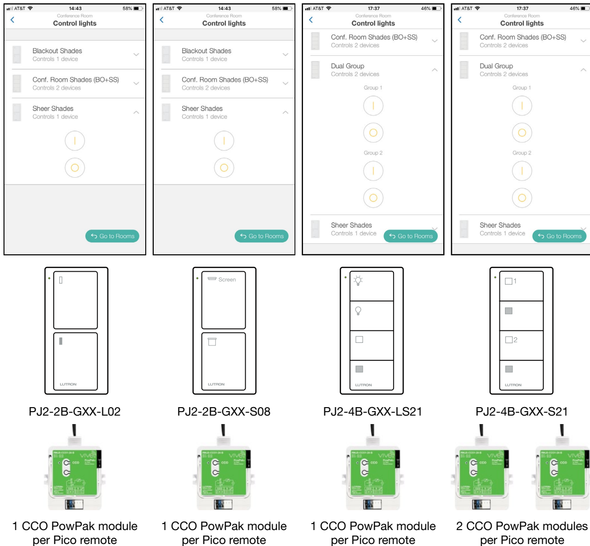
Figure 7: Inverted Shade Function (Operation of Configuration 2.2)
