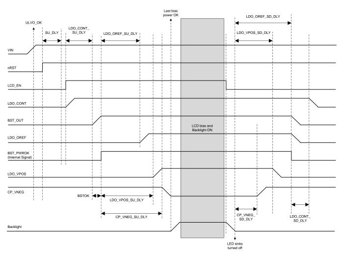
Figure 50. General LCD Bias Power Sequence With Backlight
