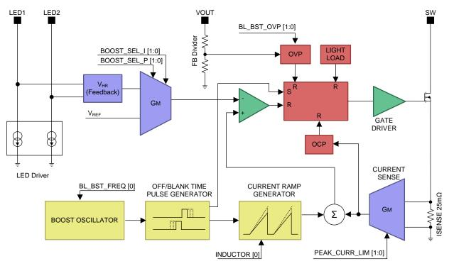
Figure 46. Backlight Boost Block Diagram
