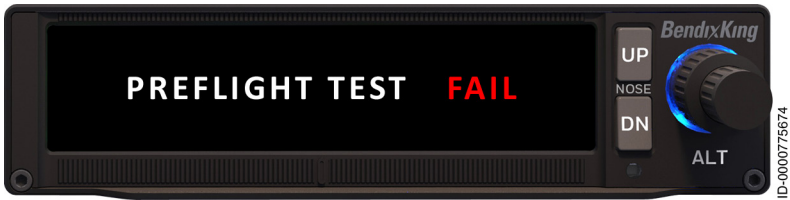
Figure 7 KFC 230 Failed Preflight Test
