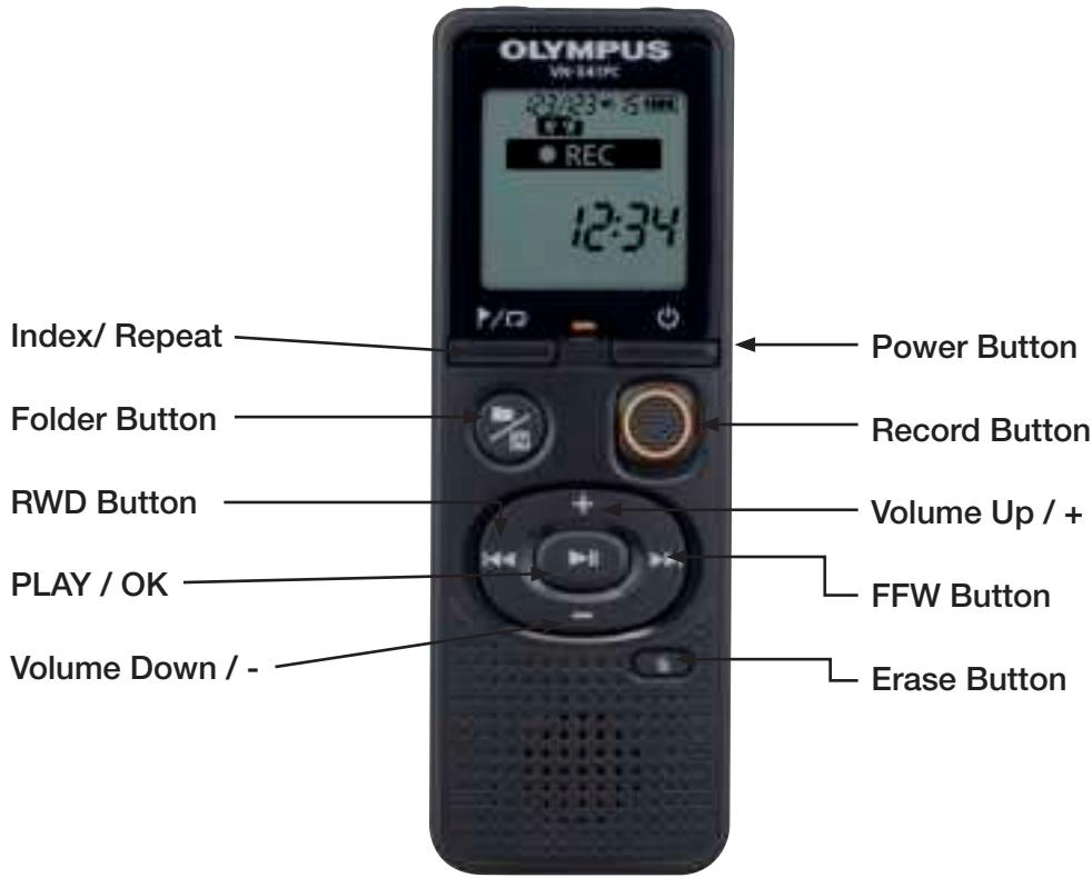
To turn on the VN-541PC press and hold down the Power button located under the power symbol until the recorder powers on. You will need to do the same thing to turn the recorder off.
