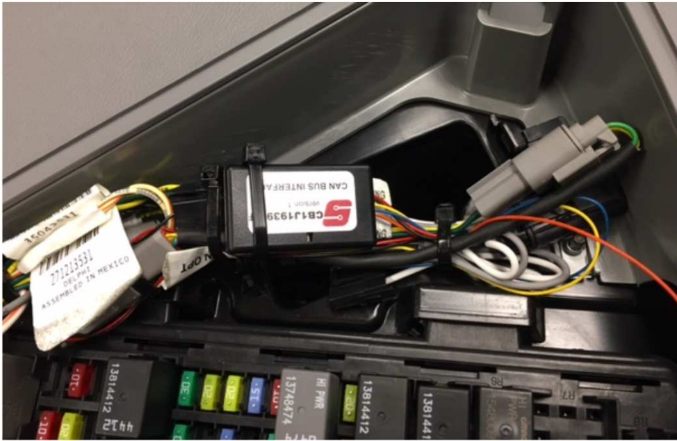
Fig. 43 CAN Bus reader installed
