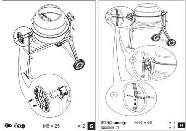
**NOTE** - The wheel must be allowed to pivot about the bolt, so that the lugs on the bracket can be engaged or disengaged from the slots in the locking plate.
