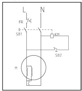
NOTE: A built-in thermal protector is arranged in the motor to prevent it from overheating. The thermal protector restores automatically when the motor cools down.
