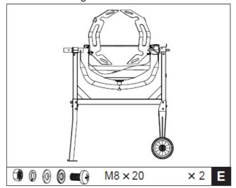
**NOTE:** Two arrow labels are affixed on the upper drum and bottom drum to assist you in lining them up to one another. If you have any difficulty in correctly positioning the mixing blades, it is helpful if you temporarily mount the upper drum on the top of the bottom drum, rotating it so that the two arrows line up.
