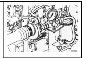
peak power and rated speed. Wait for the blowby measurement to stabilize before taking a reading.
