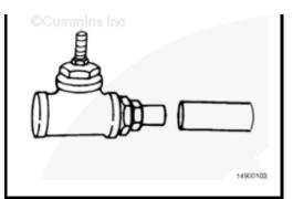
To measure the crankcase blowby pressure, connect a water manometer, Part Number ST1111-3, pressure gauge, or transducer to the blowby measurement service tool.
