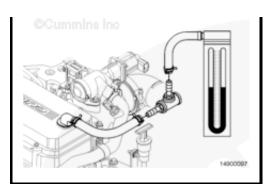
For ISB CM2150 engines that have the crankcase ventilation filter located at the rear of the engine, use the following steps to connect the blowby measurement tools.
