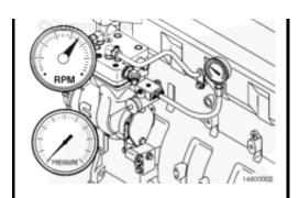
Determine the air compressor blowby pressure contribution by determining the difference in the blowby pressure measurement with the air compressor pumping and the air compressor **not** pumping.
