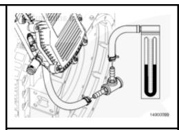
For ISC and ISL CM2150 and QSL CM2250 engines, use the following steps to connect the blowby measurement tools.
