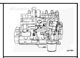
Close the valve (A) that allows oil to drain into the bucket.
