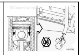
The tools used to measure blowby are similar in design. The difference between the tools is in the size of the orifice. Different size orifices are available to more accurately measure blowby by accommodating the wide variety of engine configurations and ratings. This is due to the fact that engine blowby is dependent on the volume of intake airflow.
