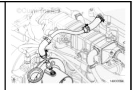
If the crankcase ventilation line is connected to the turbocharger housing, install a straight thread plug, Part Number 3089567. Plug the crankcase ventilation line with a suitable fitting.
