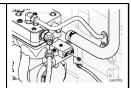
To unload the air compressor, determine the pressure needed at the governor/unloader air signal port to start and stop the air compressor from pumping.
