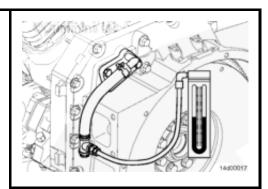
systems with crankcase ventilation filters, follow the proceeding steps on connecting the blowby measurement equipment.
