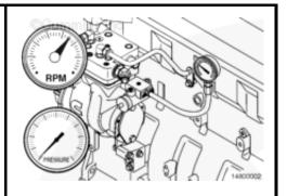
determine when the air compressor will stop pumping (system pressure stops rising at this point). Record the signal line pressure.
