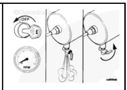
system down by opening the drain cock on the wet tank to release compressed air from the system.
