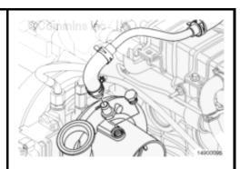
Remove the oil fill cap from the rocker lever cover. Install an oil fill adapter, Part Number 3990099.
