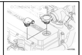
Connect the appropriate blowby service tool to the outlet of the oil fill adapter.
