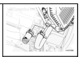
Connect the appropriate blowby service tool to the crankcase ventilation line exiting the flywheel housing. Connect a water manometer, pressure gauge, or transducer to the blowby service tool.
