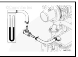
Use a suitable fitting to plug the crankcase breather tube.
