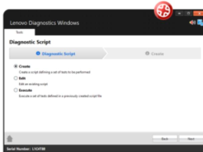
**Warning:** When the user executes a script, unsupported tests on the machine will receive the status – **NOT APPLICABLE**.
