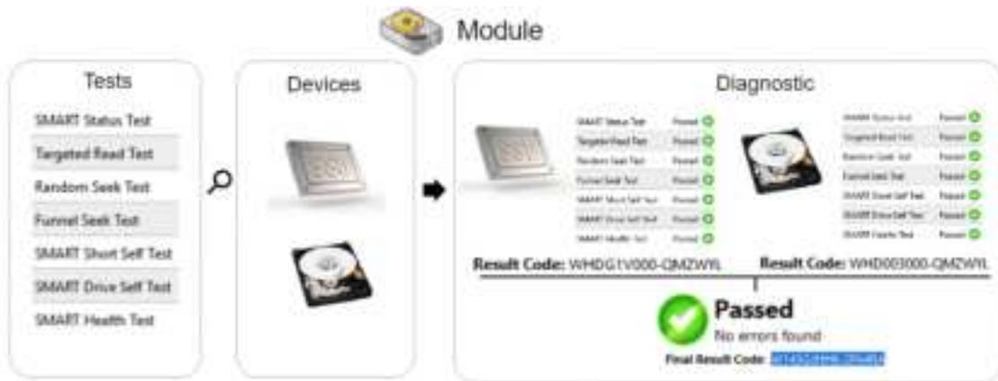
When a diagnostic is finished, Lenovo Diagnostics displays the results for each performed test and create two results codes resuming the test execution.
