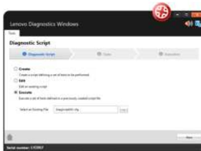
By selecting a valid diagnostic script file and clicking on the Next button, a screen is displayed with the configuration from the selected diagnostic script. All selected tests are listed selected and the not supported one are marked with the icon
