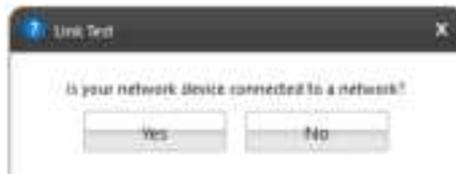
The test is performed according to the user answer. If the user selected "Yes", the test tries to establish a network link and if the user select "No" the tests verifies if the device has, indeed, no network link.
