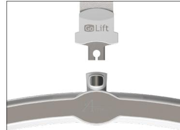
2. Insert the strap attachment in the slot on the Carry Bar top cover with the open side facing down and release the button.
