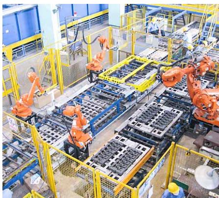
Robots operating in a sand core cell on a cylinder heads manufacturing line in China.
