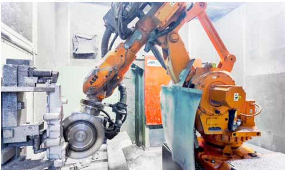
The adaptive motion controller adjusts the behavior of the IRB 6660 in response to the forces it encounters.
