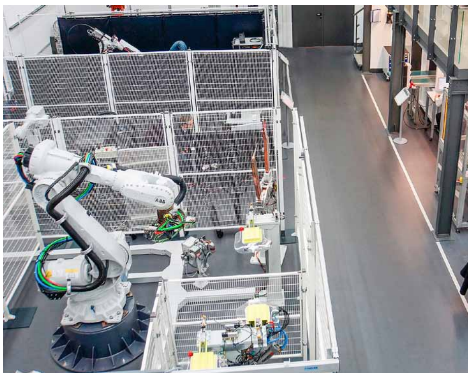
Robots operating in a sand core cell on a cylinder heads manufacturing line in China.
