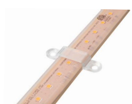
Mounting Clips – Provide secure attachment to a variety of surfaces when placed at 1-foot intervals. The back of luminaires features 3M adhesive strips to maintain positioning while installing clips.
