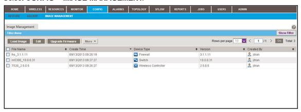
**5.** To add columns to or remove them from the Image Management table, right-click the table heading anywhere, and specify the columns by selecting the corresponding check boxes.
