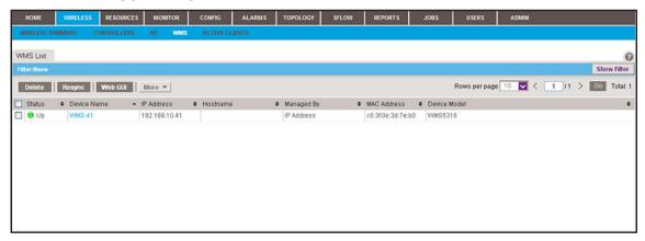
**5.** To add columns to or remove them from the WMS List table, right-click the table heading anywhere, and specify the columns by selecting the corresponding check boxes.
