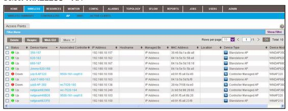
**5.** To add columns to or remove them from the Access Points table, right-click the table heading anywhere, and specify the columns by selecting the corresponding check boxes.
