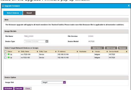
The Select Devices pop-up window closes and the selected device or devices are listed on the Upgrade Firmware pop-up window.
