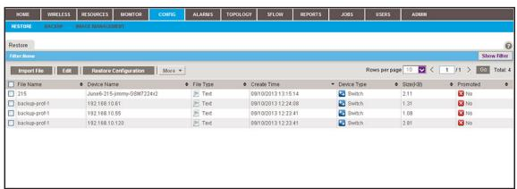
**5.** To add columns to or remove them from the Restore table, right-click the table heading anywhere, and specify the columns by selecting the corresponding check boxes.
