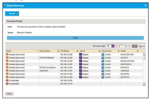
**Note:** If a credential failure occurs, a common reason is that the device login information changed from its default. When a credential failure occurs, add or modify the credential and run the discovery job again. For more information, see Add a device credential on page 35.
