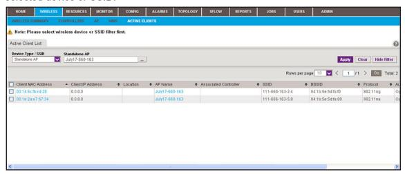
**12.** To add columns to or remove them from the Active Client List table, right-click the table heading anywhere, and specify the columns by selecting the corresponding check boxes.
