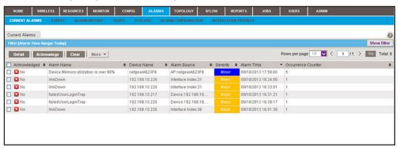
**5.** To add columns to or remove them from the Current Alarms table, right-click the table heading anywhere, and specify the columns by selecting the corresponding check boxes.
