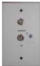
Antenna Power Supply
