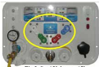
Fig 2: Set 4 Valves to 45°
