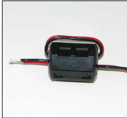
Figure A-3 EMI Filter Installed
