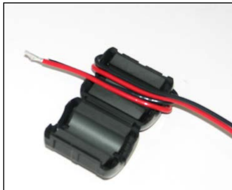
Figure A-2 EMI Filter Installation (showing wire loops)
