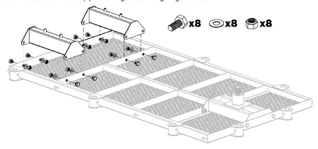
**Step 3**Attach the rear axle to the rear axle mounts. Finger-tighten nuts.
