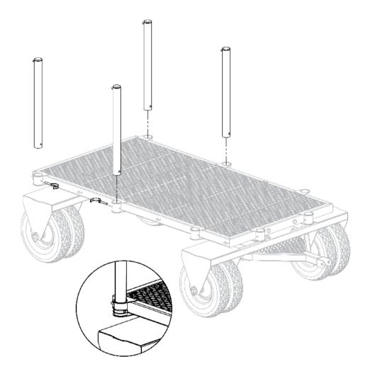
**Step 9**Attach the front posts (2) and the front panel (1) to the wagon. Secure using the locking pins.
