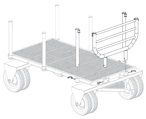
**Step 10**Attach the chains (2) to connect the front posts and front panel to the wagon. Tighten bolts securely.
