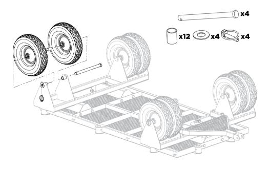
**Step 7**Tighten all nuts and bolts securely then flip the wagon onto the tires. Team lift is recommended.
