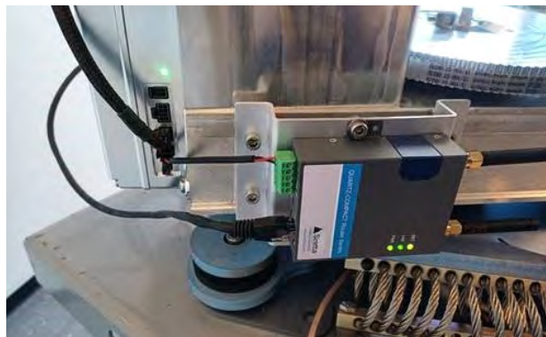
Figure 2-24: LTE modem connection, example
