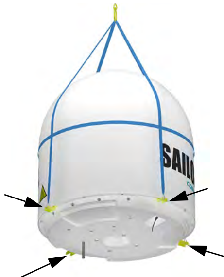
Figure 2-15: ADU installation, webbed sling attached to the 4 lifting brackets
