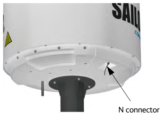
Figure 2-17: Connecting the ADU cable
