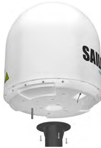
Figure 2-16: Mounting the ADU on the mast flange
