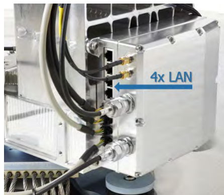
Figure 2-21: ACM LAN ports
