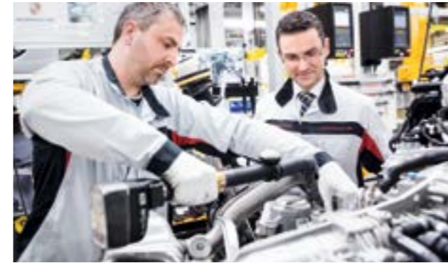
The wireless EC-screwdriver with tracking system is an important innovation in vehicle assembly.
