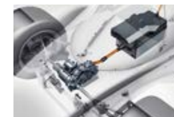
> 400 hp The Single Electric Engine provides its power on demand via a differential on both front wheels. The state-of-the-art battery power centre is positioned in the centre of the vehicle.
