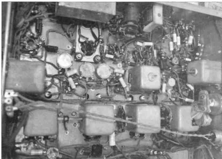
Bottom view of the chassis after most of the capacitors were replaced
