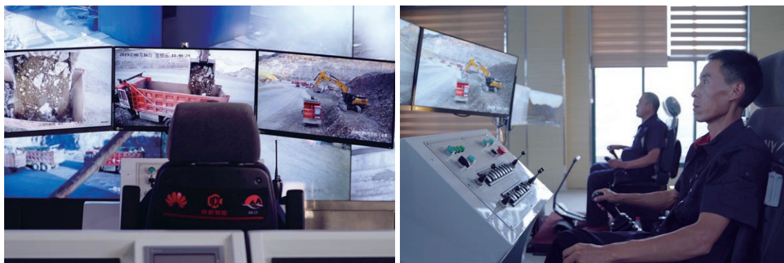
China Molybdenum workers remotely operating an excavator over a 5G network
